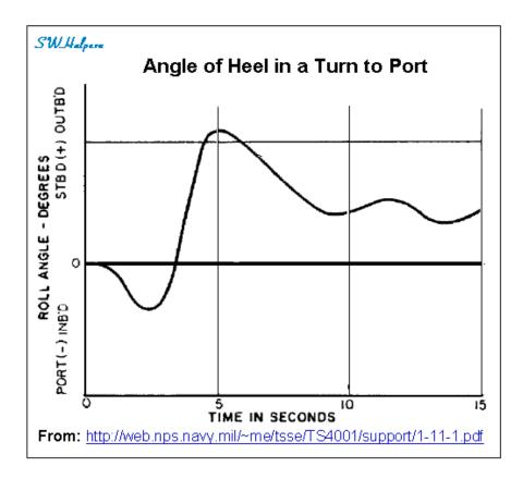
For *Titanic* in a steady-state, full-speed turn with hard over helm, the heel angle is estimated to be about 6°. This condition is shown below for *Titanic*, and is derived in Appendix B.
