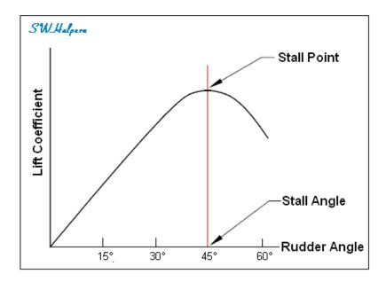
The maximum angle to which most rudders are put is about 35° to either side of the ship's centerline. *Titanic's* rudder, however, could be put over to 40° which is getting very close to the rudder stall point, the point beyond which the rudder produces less lift but significantly increasing drag.
