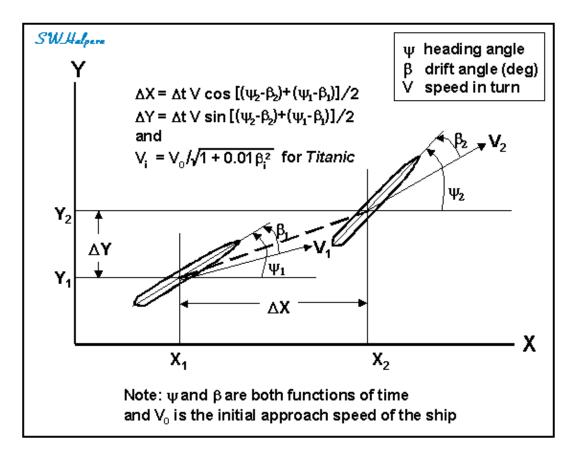
As we have discussed before, the ship's speed will decrease as the turn develops because of the increased drag on the hull that starts to build up as the ship enters a turn. For *Titanic* we found that the steady-state speed will be about 0.775  $V_0$ . Therefore we should see the speed drop from  $V_0 = 22.5$  knots to V = 17.44 knots (or 29.45 ft/sec) after the turn is fully developed. As
