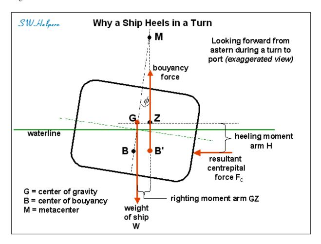
The displaced center of buoyancy in turn creates a righting moment of  $GZ \times W$ , where GZ is the righting arm equal to  $GM \sin \phi$ , and W is the force of buoyancy which must equal the ships displacement weight in tons. For relatively small angles of heel, the righting moment is therefore given by:
