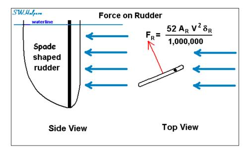
For *Titanic* running at 22.5 knots, and a full rudder deflection angle of 40 degrees, the force calculates out to 423 tons. Since the underwater area of the rudder works out to be about 402 sq. ft., this force would create a pressure of about 1.05 tons per square foot on the rudder plate.
