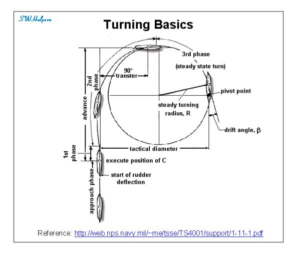
The path taken by a ship during a turn is shown in the diagram below.
