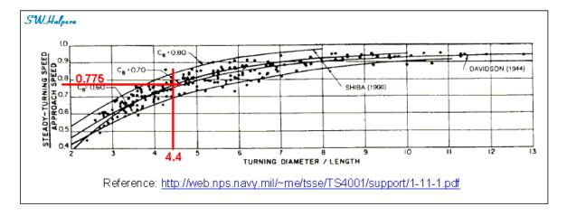
With the ship turning at about 17 knots in a 3,750 foot diameter circle, the steady-state turning rate calculates out to 9/10 of a degree per second, or just under 7 minutes per 360° turn once the ship reaches the steady-state phase.
