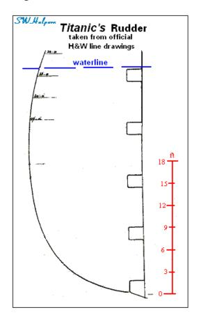
As seen in the photograph and in the drawing, *Titanic's* rudder was essentially a flat plate having somewhat of a spade shape in underwater profile. For a spade-shaped rudder working behind a ship's propeller, the force,  $F_R$ , acting on the rudder when it is deflected at an angle  $\delta_R$  to the slip stream of the water is given approximately by:<sup>27</sup>
