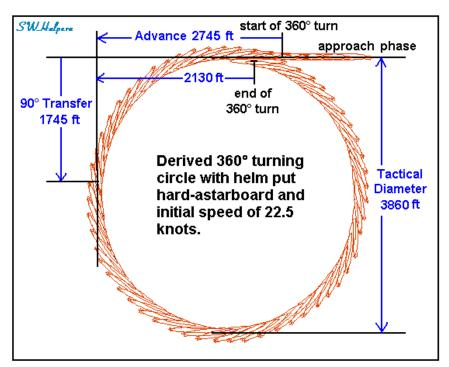
The following diagram is a more detailed plot of the ship's CG point taken in 2.5 second increments. The scale shown is 500 feet per division.
