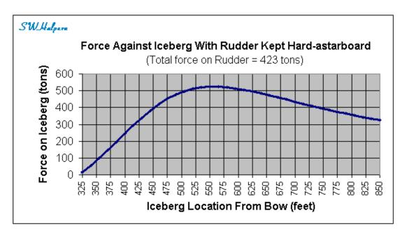
The combined forces of rudder and iceberg sets up a turning moment to port which peaks when the berg is about 375 feet aft of the bow, and then decrease to zero when the berg is alongside the stern where the lifting force of the rudder is exactly cancelled by the force of the iceberg on the hull at that point.
