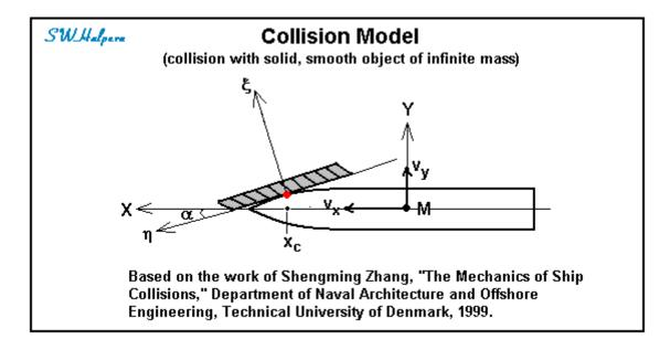
The notations and equations used for all the calculations come from the 1999 thesis of Shengming Zhang, "The Mechanics of Ship Collisions." In this case we use the scenario of a ship striking a rigid object that is smooth so that we are presented with a sliding case; i.e., small coefficient of friction.
