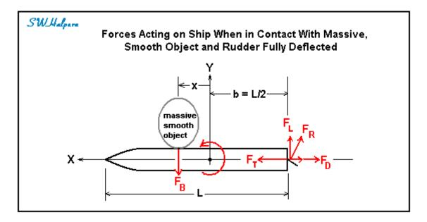
In the above we show several forces acting on the hull of the vessel,
