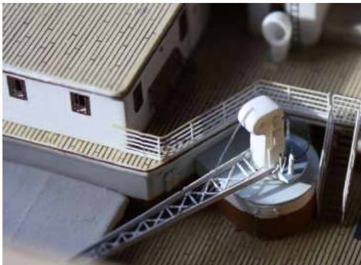
Photo of the after Well Deck of Art Braunschweiger's partially completed model, starboard side, showing photoetched brass crane jibs, ladders, handrails and benches .
